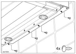
Secure the spacer strip to the back of the appliance from behind using 4 plastic rivets as shown.
